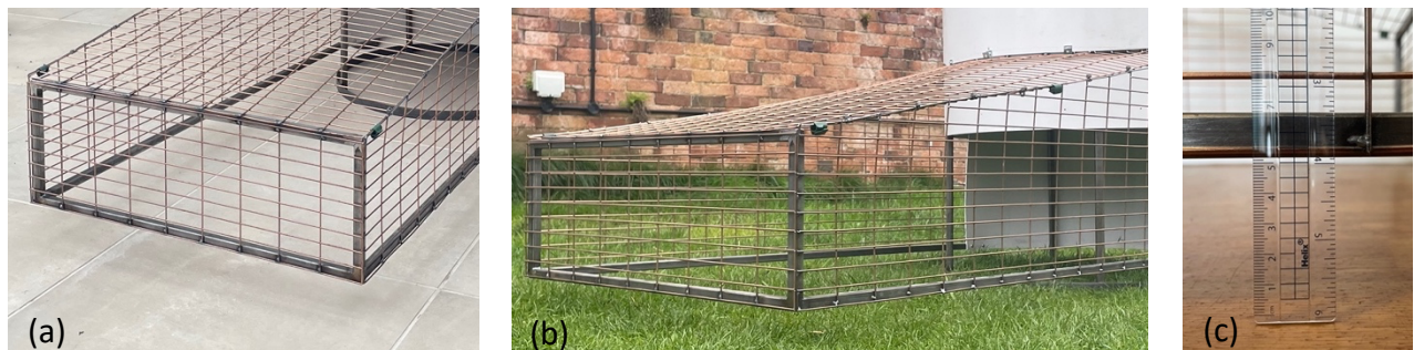
Figure 19 - Images of Full-Scale Prototype in the Upper Position, (c) shows Ruler Measurement of Height at End of Cage
