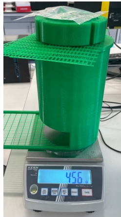
Figure 15 - Image of the weighing of the Outside Structure to be Lifted by Springs
