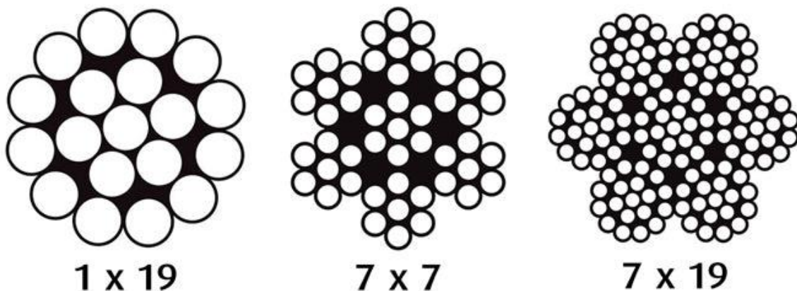
Figure 15 – A diagram showing the different strand designs of cables [5]
