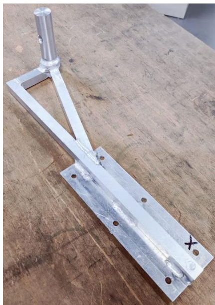
Figure 70 – An image showing the improvised solution for the base anchor point.
