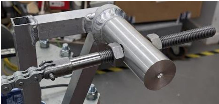
Figure 57 – An image of the chain anchor connected to the base anchor with two bolts. The chain can be tensioned by adjusting the position of the two bolts.
