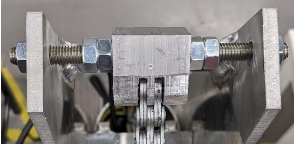
Figure 56 – An image of the chain block with the bolt spanning the whole width of the hinge.
