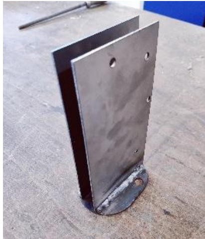
Figure 66 - Welded Steel Raceway
